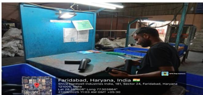
All parts undergo a 100% inspection by our inspectors, who conduct thorough visual and dimensional testing to ensure compliance with customer requirements and internal quality standards. This inspection ensures that each part meets the specified criteria before advancing to the final stage of the manufacturing process.
